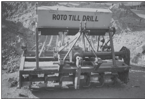
Fig. 3.12 : Roto Till Drill—A modern agricultural equipment
