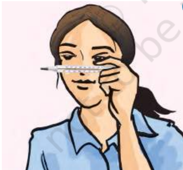
Fig. 3.3 Correct method of reading a clinical thermometer
