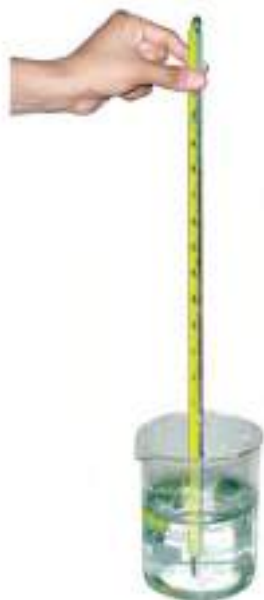
Fig. 3.5 Measuring temperature of water with a laboratory thermometer
