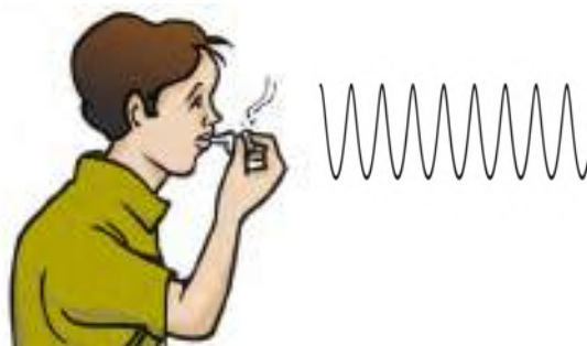
Fig. 10.18 : Frequency determines the pitch of a sound
