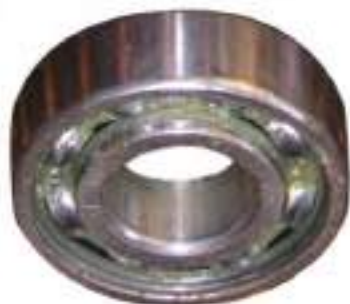
Fig. 9.16 : Ball bearings reduce friction
