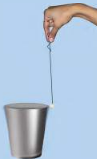
Fig. 10.17 : Thermocol ball touching the vibrating glass tumbler
